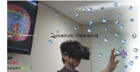
3D Finger CAPE [5] aims to infer an occluded fingertip position as well as clicking action from a single-depth sequence.
